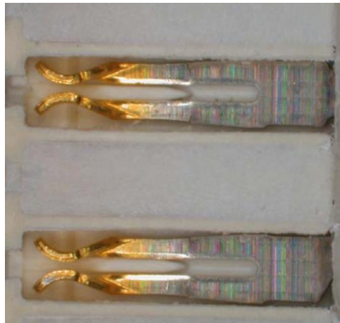
“Cross-Section of CompactPCI® Bifurcated Socket Tines (Diane Kolos, NASA/GFSC). Magnification is 8x.”
